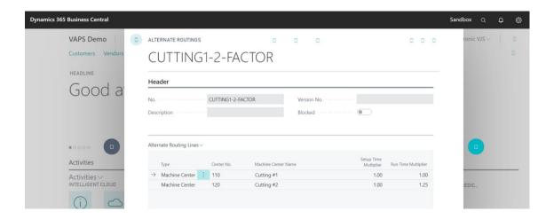
Coming back to the example we can see the first cutting machine center with a run time multiplier defined as 1.00, while the alternative machine center with a run time multiplier of 1.25.
