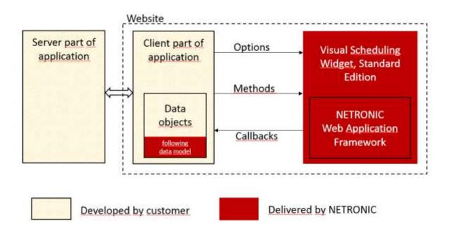
All parts of the data objects that must follow our Resource Planning Data Model, the options, the methods, and the callbacks are part of the application programming interface (API) and can be accessed by the application on client side.
