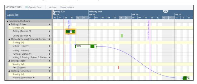
In the Availability View, the VAPS even provides an optical warning, if you drag an operation to a point of time that is before its EMAD by showing the according operation in red:
